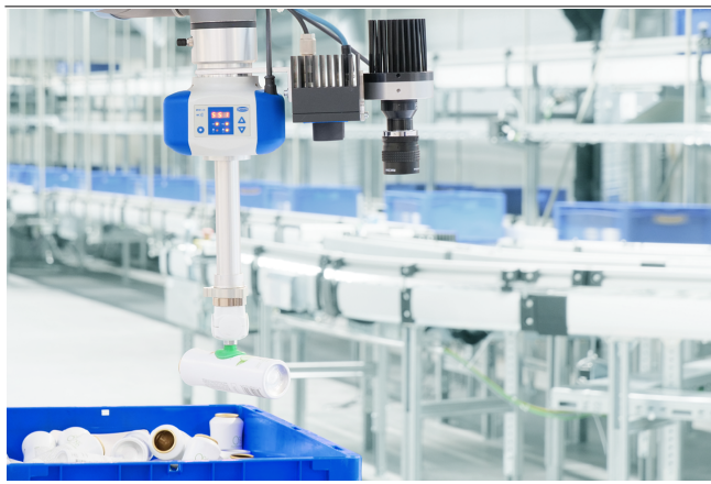
Vision & Handling Set 3D-R when handling cans
